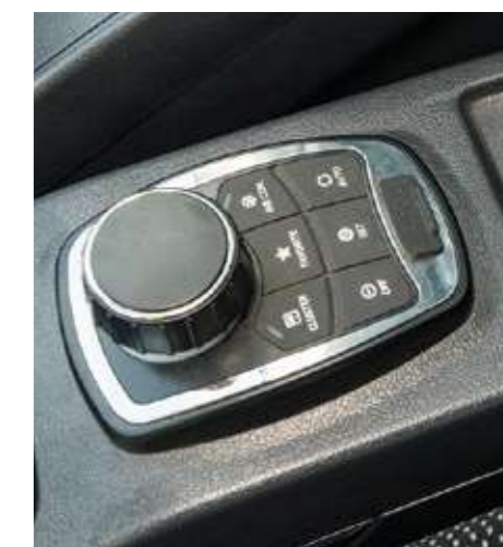
Jog dial module For added convenience, an integrated jog dial module allows easy control of the air conditioning and instrument cluster navigation.
