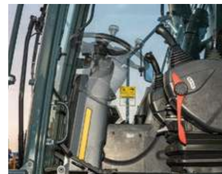
3-way adjustable steering column The steering column is ergonomically positioned and adjustable so that every operator can work more comfortably and productively.
