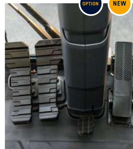
Auxiliary joystick and pedal control A 2-way proportional auxiliary joystick and pedal control enable effortless operation to minimise operator fatigue.
