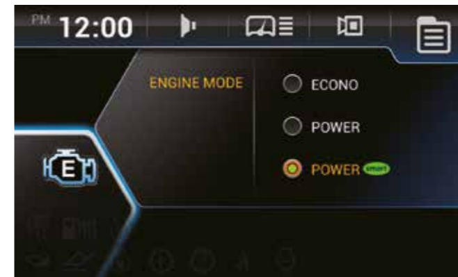
The new Smart Power mode adjusts engine RPM in heavy load work like digging to save fuel without compromising on performance. The technology also achieves an optimal balance between traction and breakout forces.
